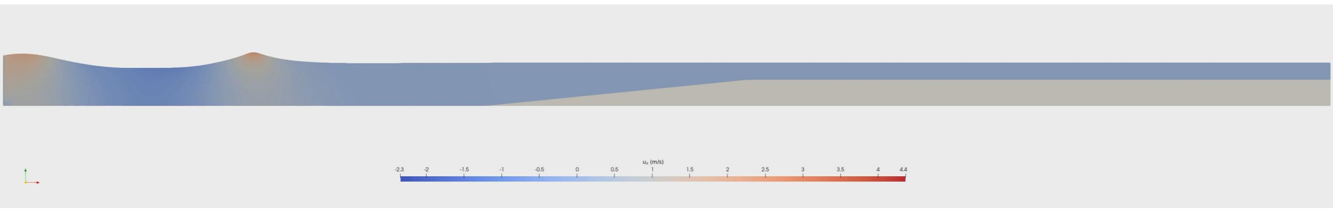
100 s of simulation in 294 s on 8 procs laptop, 41760 cells
